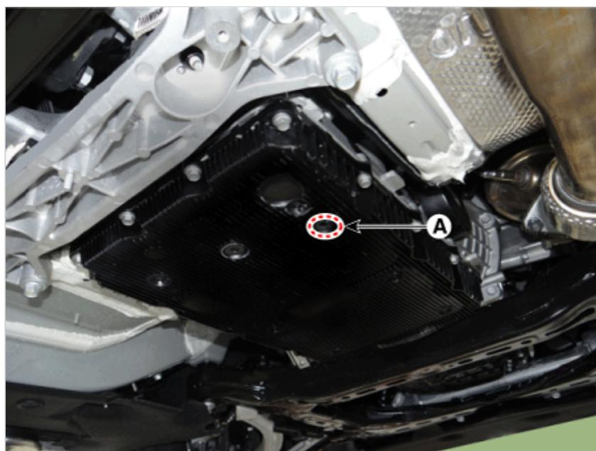
7. After ATF level check or exchange, be sure to remove ATF from outside automatic transmission.
